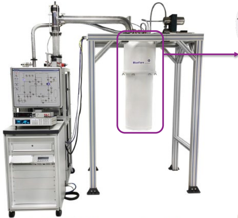
Control Unit, Gas Handling System, and cryostat in mounting frame.
